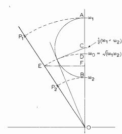
Fig. 18. Pole positions for 2nd-order band-pass response.
