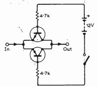
Fig. 1. Basic electronic switch.
