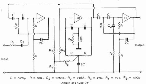
Fig. 16. 3rd-order b-p active ladder filter using parallel-T circuits.
