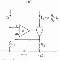
Fig. 8 (a) Current Source using 0 p. amp. and active device. (b) Terminal identification for general active device of 8(a). (c) Circuit for obtaining precise current ratio. amplifier theory that if  $A \ge l$  and commonmode effects are neglected,
