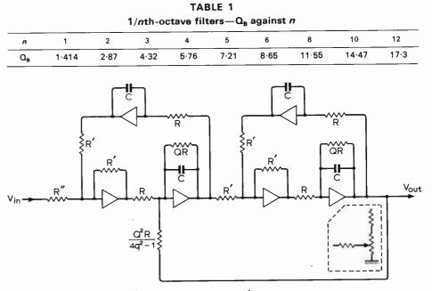
Fig. 9. 2nd-order band-pass filter using two-integrator loops.
