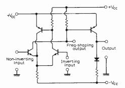
Fig. 1. Circuit of 1962 linear silicon integrated circuit (Texas Instruments SN521 operational amplifier).
