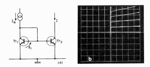
Fig. 5. (a) Integrated transistor pair in "current mirror" configuration. Emitter area ratio 1:m. (b) Current mirror characteristics using SL303A. Scales: vertical 1 mA/div; horizontal 2 V/div. Steps: 1 mA.
