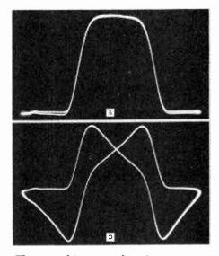
The normal input ccupling time constant of the oscilloscope is 0.25 sec. These photographs show the result of reducing it, at (a) to 0.04 sec and at (b) to 0.001sec. Notice the double trace in the vertical direction in (a) and the gross distortion in (b).
