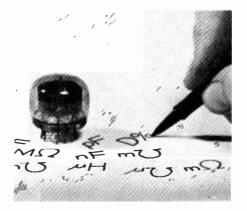
requirement is half of these figures. Base is B13B and tube height is 26.5mm. Price is about £2 for 100 up. Hivac Ltd, Stonefield Way, South Ruislip, Middx. WW318 for further details
