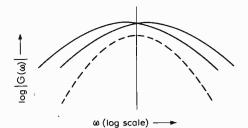
Fig. 4. Misalignment of two tuned circuits of equal Q gives a still symmetrical loop response.
