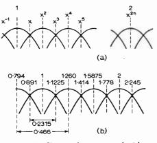
Fig. 8. (a) n filters to the octave, each with a band width of 1/nth of an octave. (b) Frequency relationships for 1/3rd-octave filters.
