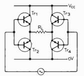
Fig. 3. Bridge output stage with the load across the d.c. null.
