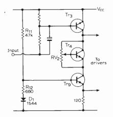
Fig. 6. Replacement of bootstrap resistor by transistor.
