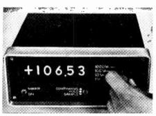
Weston standard cell. Zero offset current and voltage are automatically corrected between each reading. Series-mode rejection at mains supply frequency and its harmonics is greater than 85dB, and common-mode rejection 100dB at mains frequency and d.c. with  $1k\Omega$  imbalance in the input leads. The price is £25. International Electronics Ltd, Ewood Bridge, Haslingden, Lancs. WW303 for further details
