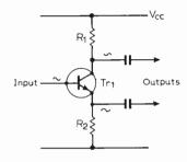
Fig. 7. Single-stage phase splitter.
