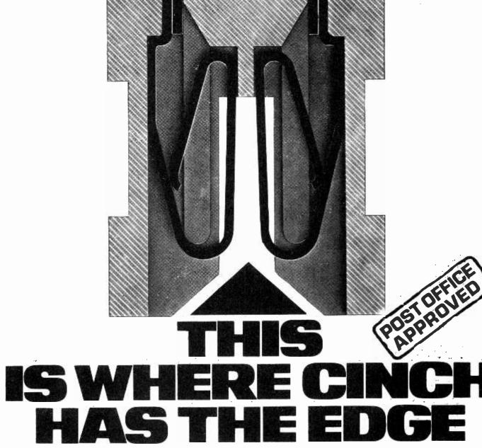
This bigger than average contact area, spring formed for extra low smooth insertion forces, is one of the major factors that gives the Cinch 0.1" Modular Edge Connector its reputation for optimum reliability. In addition, available platings include 5 microns of gold on the mating surfaces with 2 microns of gold overall.
