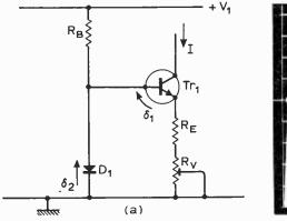
Because of the larger value of  $I_{CBO}$  for germanium transistors and the fact that  $|d\delta_2/dT| \neq |d\delta_1/dT|$  there is an increased temperature sensitivity for this configuration compared with that of Fig. 2(a).
