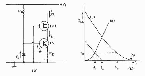
Fig. 4. (a) Improved form of circuit in Fig. 3(a). (b) Load line construction for 4(a).
