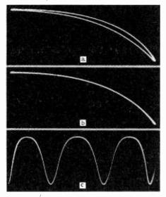
The voltage waveform at the collector of the BF177 wave shaper is shown in these photographs. At (a) the waveform is shown with a sinusoidal timebase and the double trace is due to phase shift caused by the connection of the oscilloscope. Adjusting the phase control removes this (b). The waveform with the more familiar linear timebase is shown at (c).
